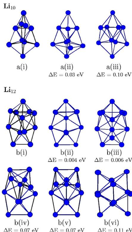
FIG. 1. (Color online) The ground-state geometry and some isomers of  $\text{Li}_{10}$  and  $\text{Li}_{12}$ . The label (i) represents the ground-state geometry. The energy difference  $\Delta E$  is given in eV with respect to the ground-state energy.
