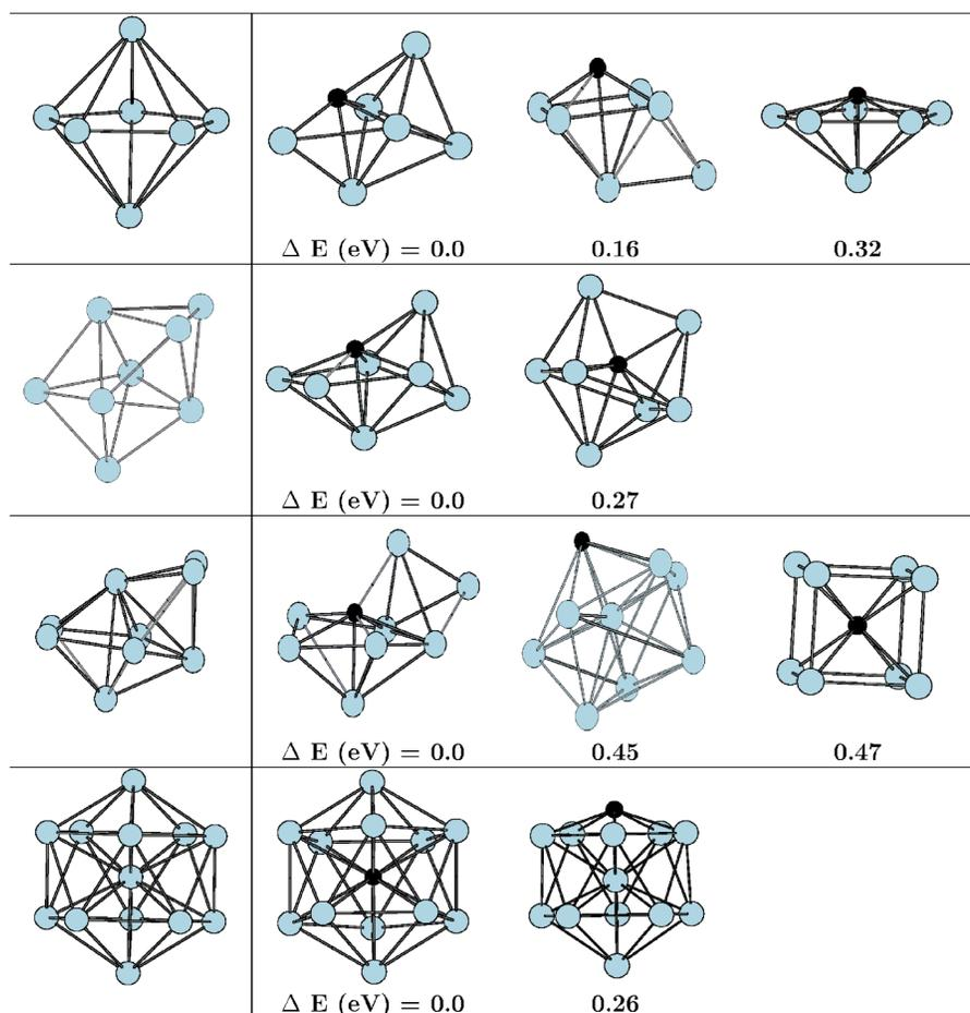
FIG. 2. Ground-state geometries of  $\text{Ni}_{n+1}$  clusters (column 1). The structures on the right side show the lowest-energy structure (column 2) and some of the low-energy isomers for  $\text{Ni}_n\text{B}$  clusters ( $n=6-12$ ). The lightly shaded spheres represent the Ni atoms and the dark sphere represents the B atom.
