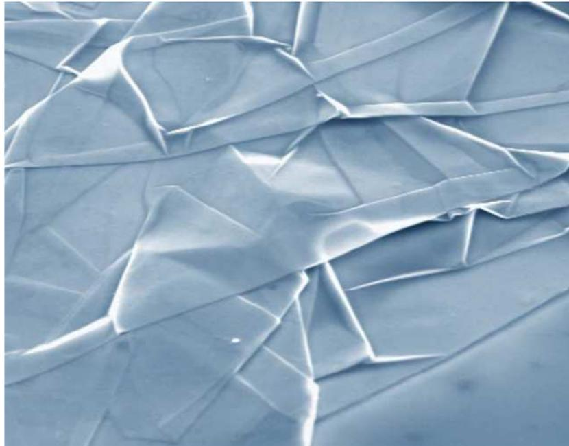
Figure 1.6 – Single atom thick sheets of graphene obtained by adhesive tapes as shown in scanning electron micrographs. (Foundation of Fundamental Research on Matter, Netherlands)
